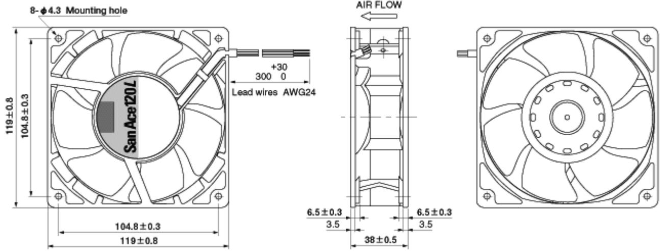
**Fig. 2 Dimensions and specifications of the low noise "SAN ACE 120L"**
