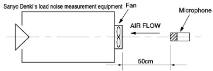
**Fig. 5 Method of load noise measurement**
