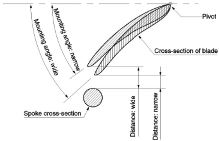
**Fig. 6 Positional relation between cross-section of blade and spoke**
