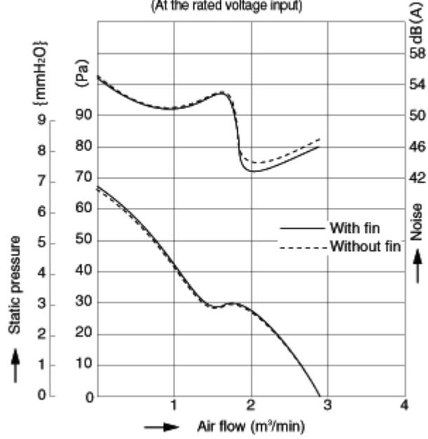
**Fig. 7 Air flow versus static pressure and noise characteristics**
