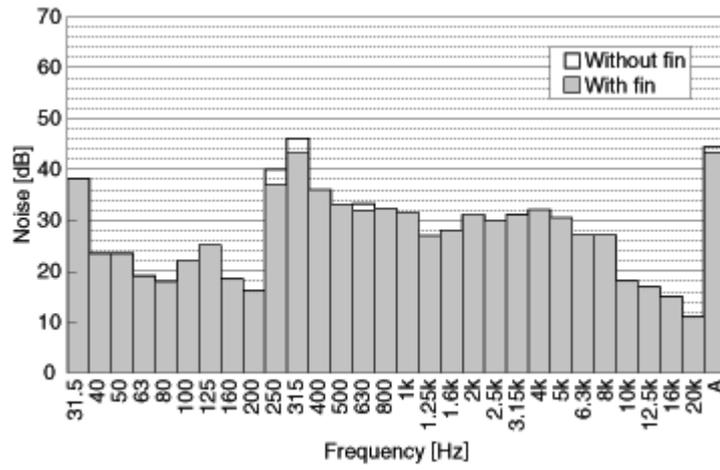
**Fig. 8 Noise analysis data of 1/3 octave band
