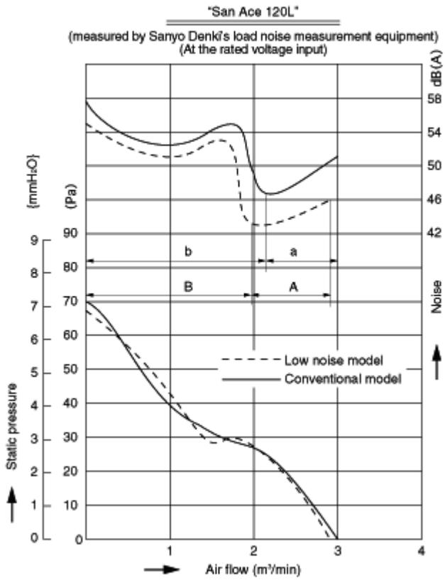
**Fig. 4 Example of air flow versus static pressure and noise characteristics**
