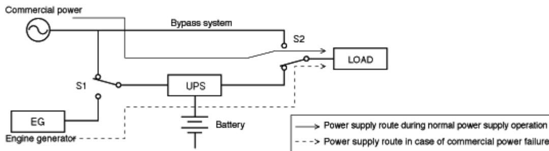
This invention relates to the UPS (uninterruptible power supply) that operates selectively on dual inputs: one is the commercial power having a large capacity and the other is an engine generator having large fluctuations of frequency and voltage. This invention is designed to improve the quality of power supplied to the load by changing the operating conditions of the UPS in accordance with the power receiving system, when overloading occurs.
