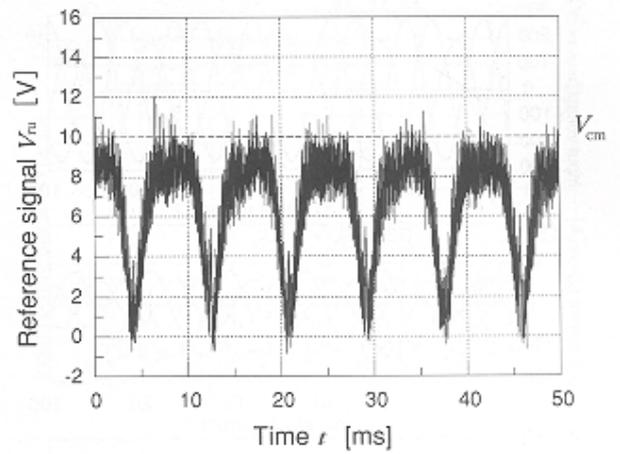
(b) Actual measured waveform of reference signal
