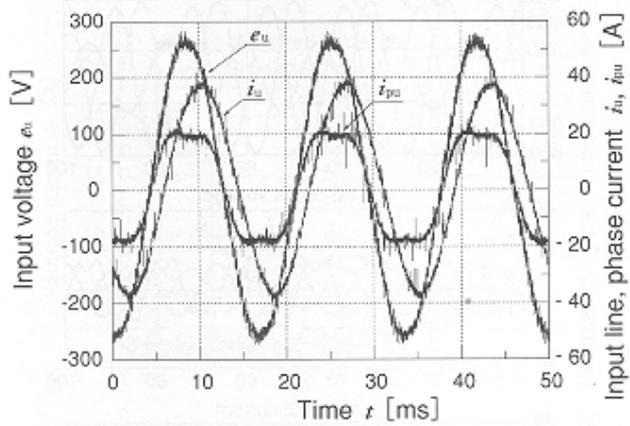
(a) Actual measured waveform of input line current and phase current
