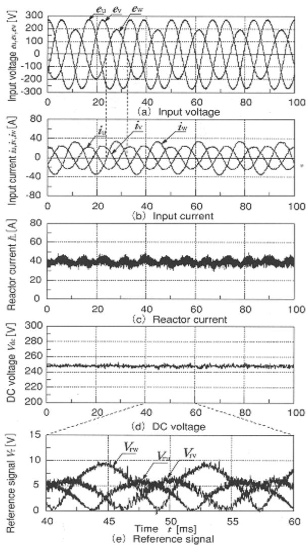
Fig. 8 Waveforms at various points when the characteristics compensation circuit is used (Unbalanced factor  $k=20\%$ ,  $E_{acw} = 100$  [V])
