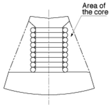
Fig.2 Rear view of the divided laminated core
