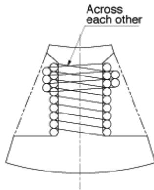
Fig.3 New type inner wire winding machine
