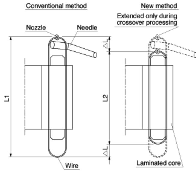
Fig.8 New work rotation type wire winding machine
