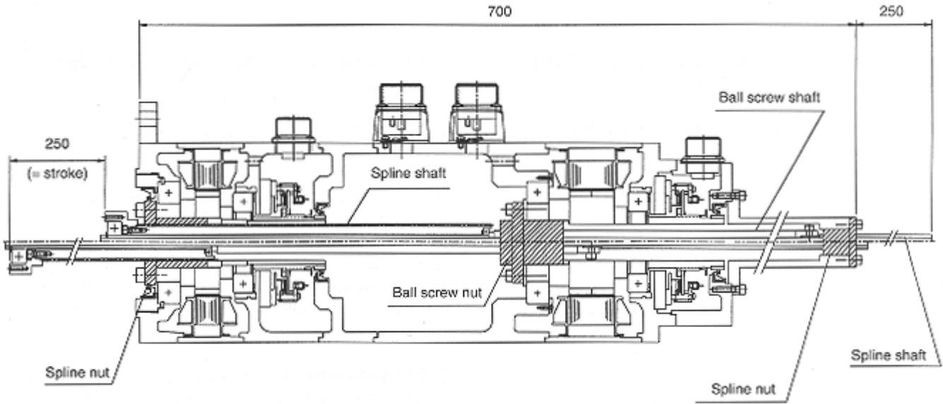
Fig.6 Cross-section of linear motion stepping motor
