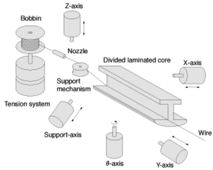
Fig.10 Process of wire winding
