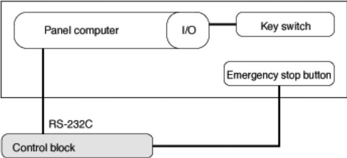
Fig.5 Software structure of the operation display block
