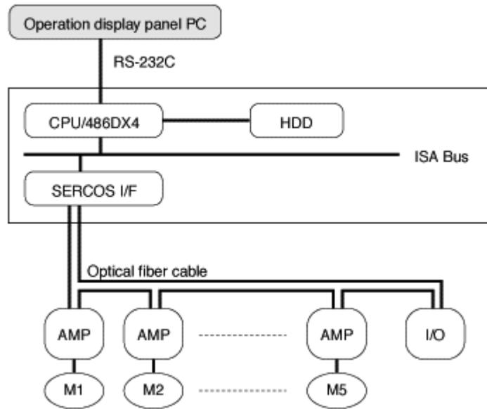
Fig.10 Software structure of the control block
