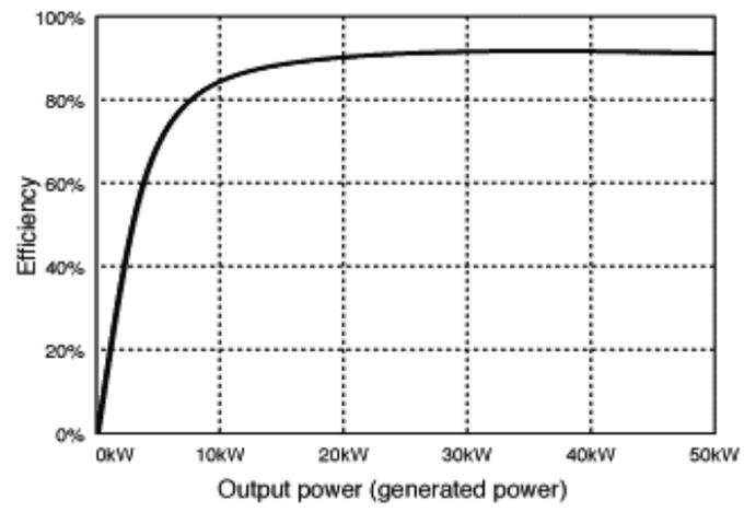
Fig.5 Running efficiency of 50kW "PMB"
