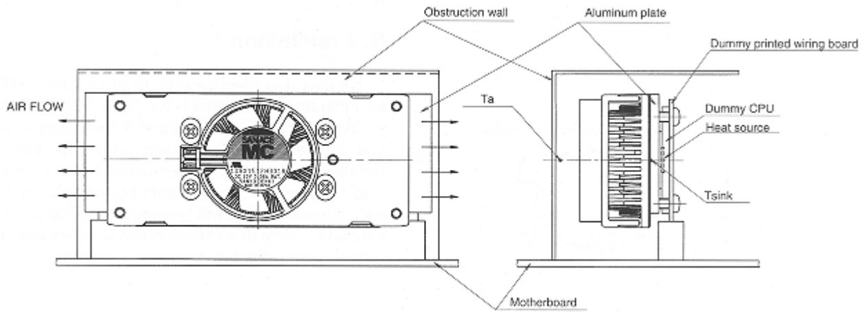
Fig.4 Air flow of an ordinary heat sink fan
