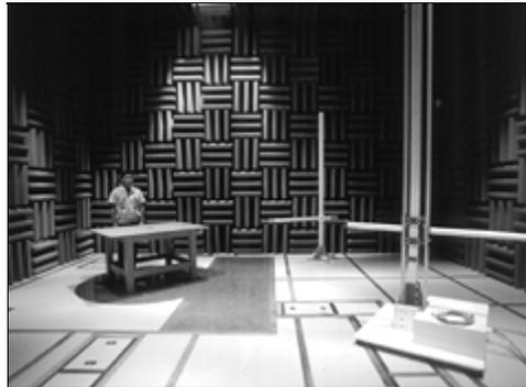
The main additional equipment of the acoustic and anechoic chamber is a turntable having the withstand load of 2 tons for a diameter of 2 m; most turntables used in acoustic and anechoic chambers are 0.5-ton class. Also, various large-capacity power supplies are installed for test pieces satisfying the requirements of 10-meter class chambers.
