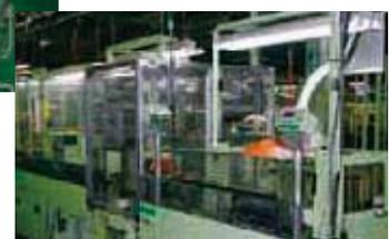
Lead-free high-temperature soldering equipment at the Fujiyama Works
