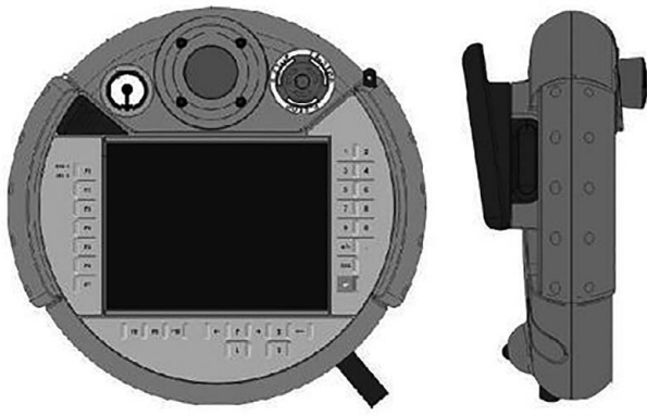
Fig. 2 External appearance of the teaching pendant
