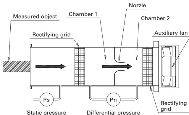
Fig. 3: Model diagram of the Airflow Tester
