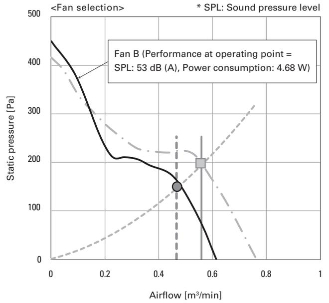
Fig. 6: Optimal fan selection from the system impedance of a device
