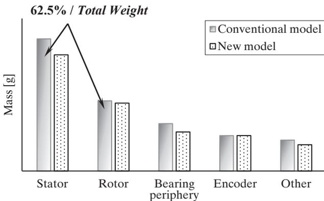
Fig. 4: Mass pallet analysis per component
