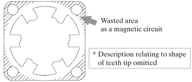
Fig. 5: Shape of the conventional model stator core
