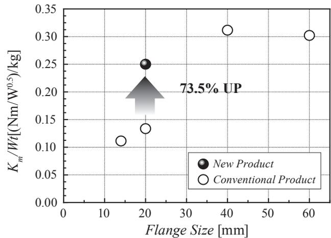
Fig. 8: Comparison of motor constant density
