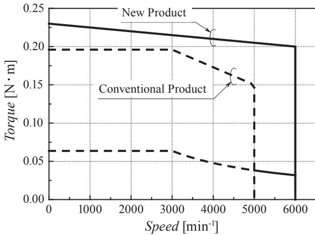
Fig. 6: Torque vs. speed characteristics (Combined with a Sanyo Denki amplifier, 48 V DC)
