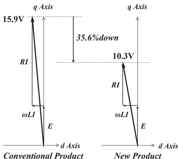
Fig. 3: Phasor diagram (N = 3000 min<sup>-1</sup>)
