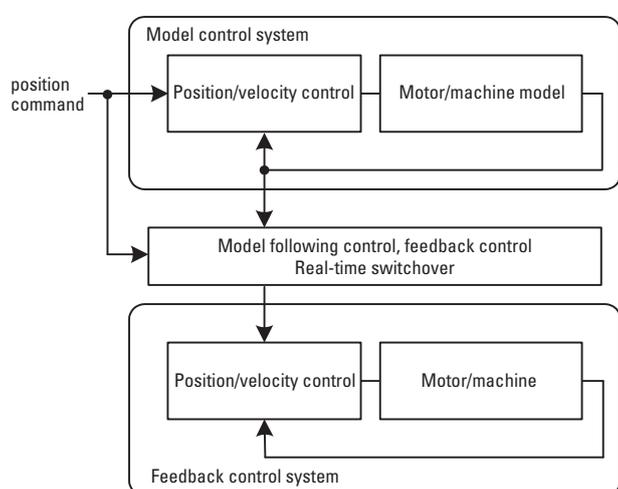
Fig. 3: Real-time switchover function for model following control and feedback control
