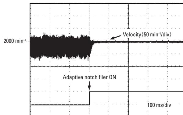
Fig. 4: Suppression of machine resonance with an adaptive notch filter
