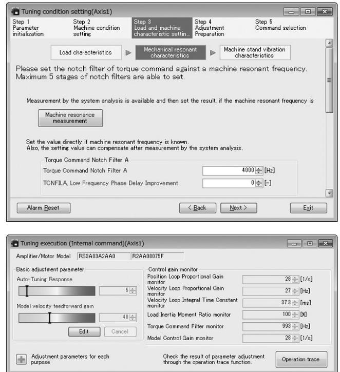
Fig. 5: Servo adjustment support function screen
