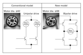
Fig.3: Comparison of size and drive system for conventional model and new model
