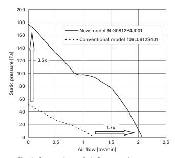
Fig. 2: Comparison of air flow - static pressure characteristics between our conventional model and new model
