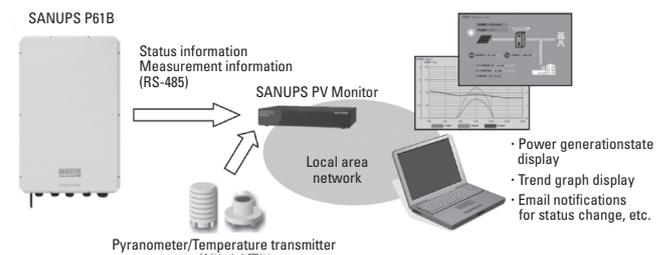
Fig. 7: Image of connection to “SANUPS PV Monitor”
