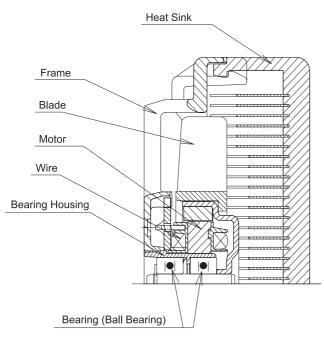
Fig.3 Structure Drawing of the "SAN ACE MC" for Pentium<sup>®</sup>4 1U Server
