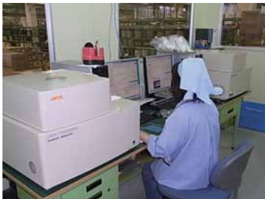
An X-ray fluorescent analysis device at the Kangawa Works
